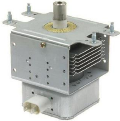
Magnétron 2.45 GHz, 1.2 kW (4.5 kV, 0.4 A, \eta = 60\% )
