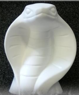
Microwave sintered of a 3D printed alumina 'snake'
